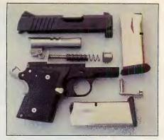
The Warthog field strips in seconds without tools. Note its supported chamber and conical barrel, and the full "beavertail" grip safety to prevent hammer bite.
